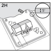
Sample 5 (2H): Lake Access (Double Loop) From the Fence Transmitter, run the wire to A, A to B, make a U-turn and go to C, C to D, D to E, make a U-turn and follow your path all the way back to A keeping wire separated at least 5 feet. Twist the wire from A back to the Fence Transmitter.
